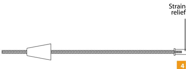
**4** Insert the coaxial cable through the flared end of the strain relief.
