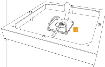
Install fixture over the brass nipple previously mounted on the wall.
