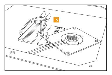
6 Screw the lid with LED Module from step 3. Ensure the ground wire is screws into the lid.
