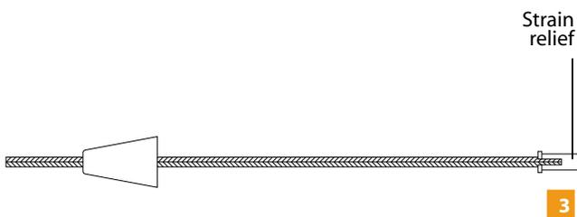
**3** Insert the coaxial cable through the flared end of the strain relief.
