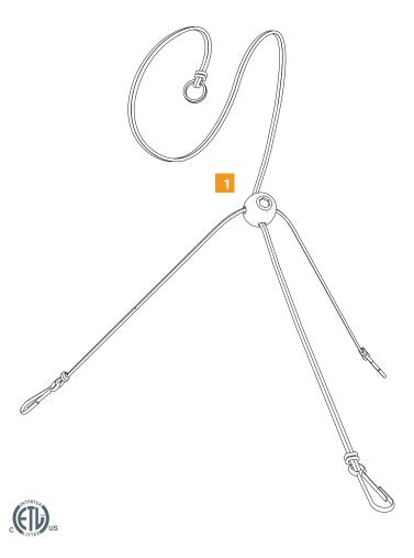
2 Stick clip from inside of glass through glass hole and pull through.
