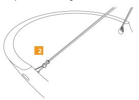
Pull gently to tighten cable around rim of glass. Center the loop on end of glass and take up any slack in cable loop.
