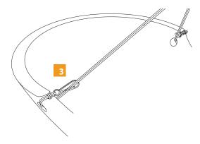
4 Take center metal ball with strain relief and center to a location in which when you hold up the cable from above the glass sits level. If it is not level all you need to do is slide the metal ball forward or back and the glass angle will change.
