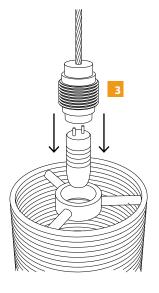
4 Line up the posts on the replacement lamp with the oval holes on the socket, and gently push the lamp into place.
