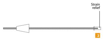
2 Insert the coaxial cable through the flared end of the strain relief.
