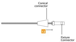
12 Slide the conical connector over the fixture connector.
