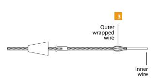
3 Slide the outer wrapped wire back to expose the inner wire.
