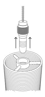
5 Screw fitter assembly into metal shade.
