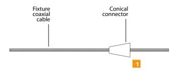
Insert the fixture coaxial cable through the conical connector
