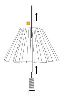
1 Feed coaxial cable as shown through applicable glass.
