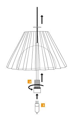
2 Rotate to raise or lower glass leveling nut. Raise or lower and fine adjust nut level so top of socket holder (threaded part) is level with top of glass.
