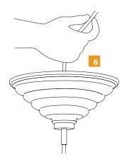
Test strain relief installation by firmly pulling on the SVT cord while bracing the coupler assembly to ensure it does not slip or move whatsoever.
