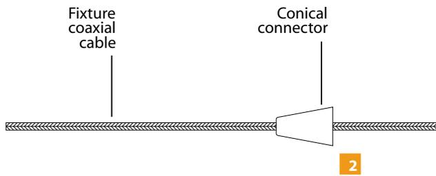
**2** Insert the fixture coaxial cable through the conical connector
