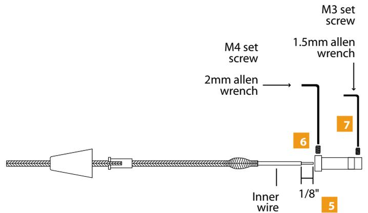
**5** Strip 1/8" from end of the inner wire. Make sure that the stripped portion is not greater than 3/16".
