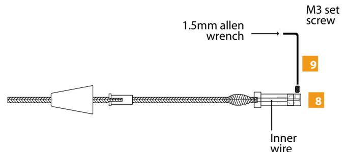
**8** While inserting the inner wire into the connector look through the set screw hole to make sure that the stripped portion of the inner wire contacts end of the connector.
